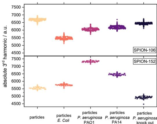
**Figure 2:** Specificity screening of antibody-functionalised SPI-ONs for *P. aeruginosa* detection.
