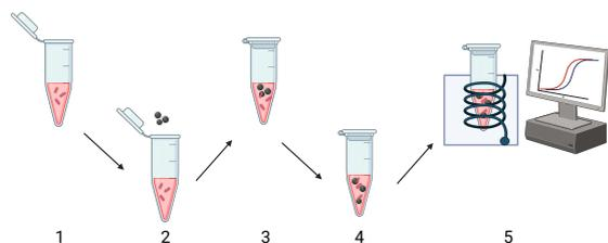
**Figure 1: MPS assay workflow.** 1 A blood sample (50  $\mu$ l) doped with *P. aeruginosa* is mixed with 2 antibody-modified SPIONs (100  $\mu$ l total volume), 3-4 incubated for 10 min, and 5 measured.
