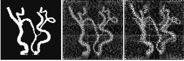
Figure 1: Simulated MPI images: software phantom (left), simulated image without object motion (center), and with circular object motion for \alpha = 5 (right).
