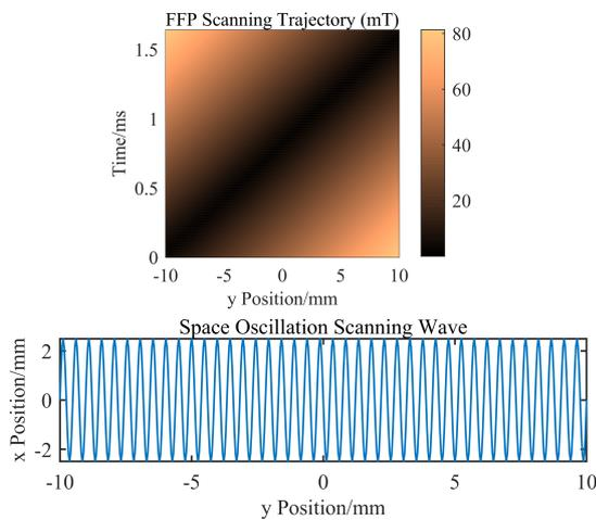
**Figure 2:** FFP scanning trajectory. FFP scans along the y direction under the action of the focus field, the 1D scan time is 1.6ms. Due to drive field, FFP oscillates rapidly in the x direction while scanning in the y direction.
