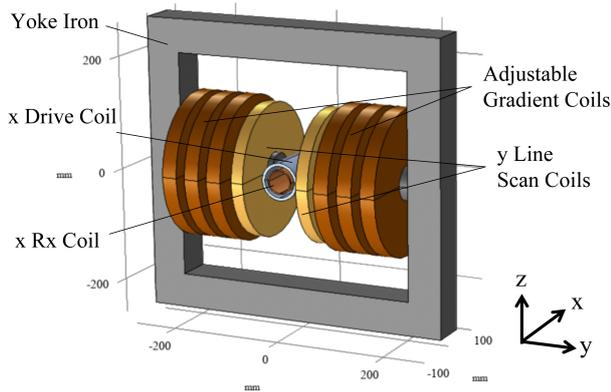
**Figure 1:** Structure diagram of HHP MPI scanner.
