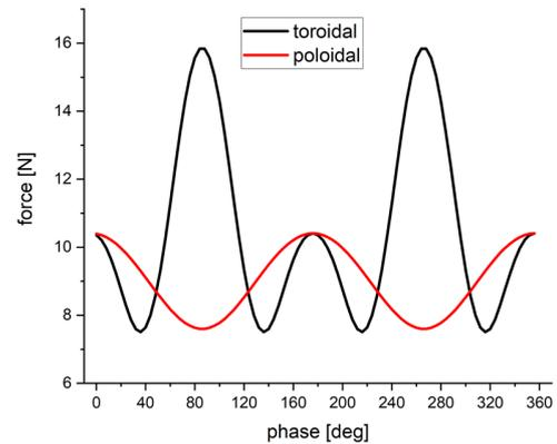
**Figure 4:** Simulation of the forces arising during a full  $360^\circ$  degree toroidal and poloidal rotation of a Halbach ring ( $k=0$ ).
