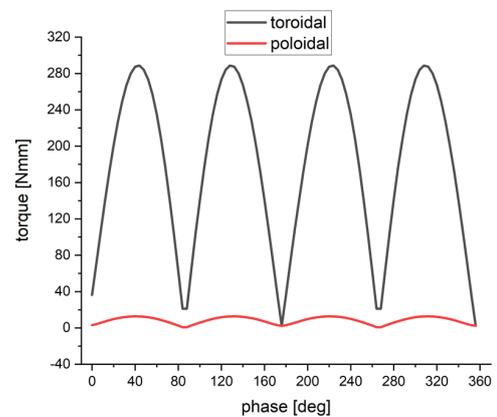
**Figure 5:** Simulation of the torques arising during a full  $360^\circ$  degree toroidal and poloidal rotation of a Halbach ring ( $k=0$ ).
