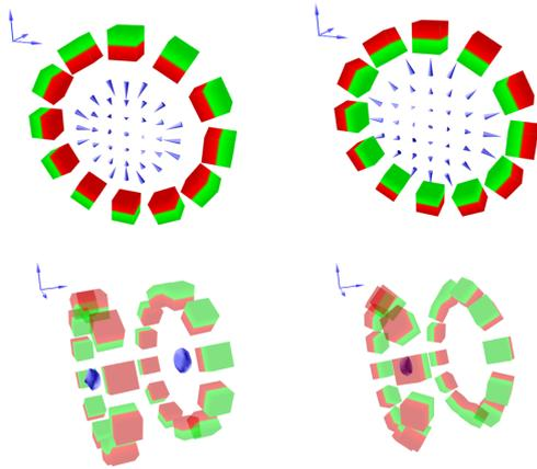
**Figure 2:** Top: two Halbach rings ( $k=0$ ) with different poloidal rotation angle. Bottom: by positioning both rings at a fixed distance and under continuous synchronous vortex rotation, two field free points (blue spheres) are generated traveling along the symmetry axis (Traveling Wave approach [9]).
