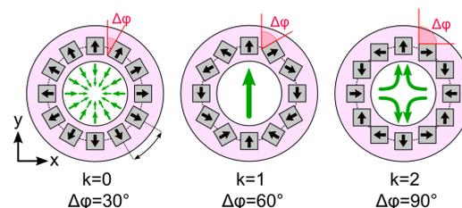
**Figure 1:** Halbach rings consist of multiple permanent magnets assembled on a ring with a specific angle generating different magnetic field configurations.
