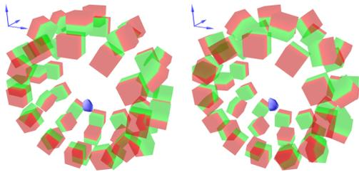
**Figure 3:** Additional Halbach rings (configuration  $k=1$ ) assembled in the center of the  $k=0$  rings and counter rotated with different frequencies  $f_2$  and  $f_3$  to steer the FFPs along a rose trajectory. Combining all rotations, a full coverage of the FOV can be reached.
