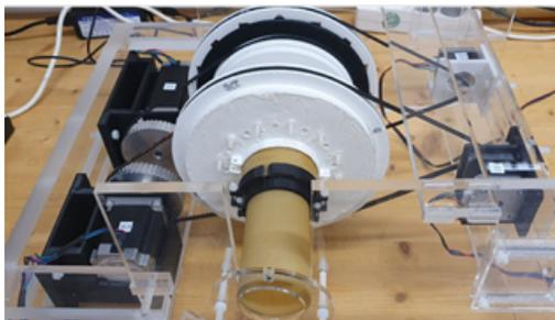
**Figure 6:** Fully implemented mechanical driven Traveling Wave MPI.
