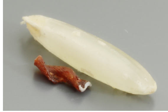
Figure 1: The magnetic microrobot has a helical Savonius shape. It is coated with SPIONs and the tip contains NdFeB particles. It is 3 mm long and therefore smaller than a grain of rice.
