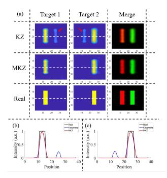
**Figure 1:** The reconstruction result in 40 dB noise level. (a): The white dot lines represent the profile lines. The red arrows point out artifacts in results. (b) and (c): The profile lines of target 1 and target 2.
