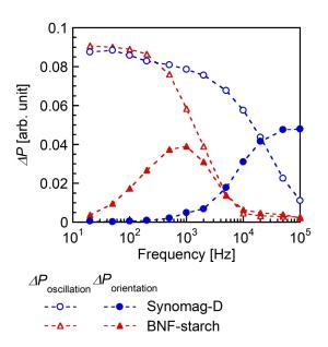
**Figure 3:** Frequency dependence of the oscillation and orientation of the easy axis under AC magnetic fields of 8 kA/m.  $\Delta P_{\text{oscillation}}$  and  $\Delta P_{\text{orientation}}$  are the degree of the oscillation and orientation of the easy axis evaluated by the optical transmission, respectively.
