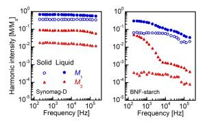
**Figure 2**: Frequency dependence of the fundamental and third harmonic intensity of magnetization under AC magnetic fields of 8 kA/m.
