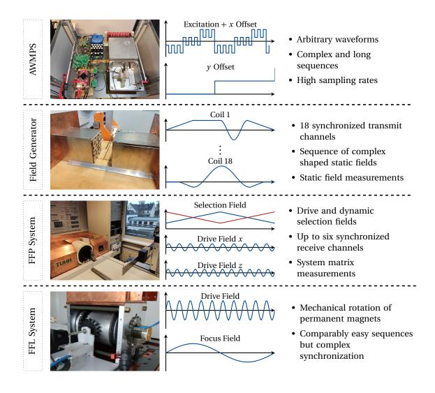
Figure 1: Systems using MPIMeasurements.jl. Each row shows a different system. The second column depicts an exemplary plot of a systems typical Sequence, while the third columns lists distinctive properties of a scanner or its operation that are covered by MPIMeasurements.jl.
